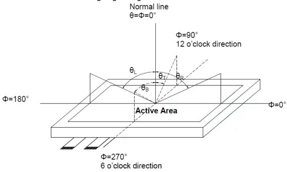
Note 2 : Definition of optical measurement system.
